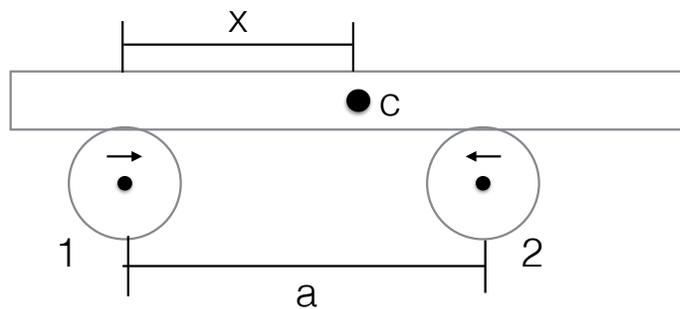
a)(7 pts) The rollers are rotating as shown in the figure and there is a coefficient of friction of  $\mu$  between the rod and the rollers. Give the equation of motion for the rod and solve for the displacement  $x(t)$  of the center of the rod  $C$  from roller 1 assuming  $x(0) = x_0$  and  $\dot{x}(0) = 0$ .
