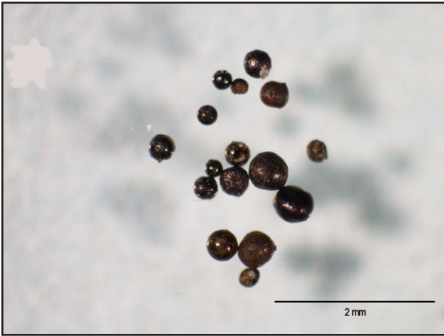
Very fine sand-sized microspheres comprised of magnetite in fly ash-impacted urban soils in Detroit.
