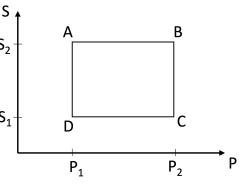
(a) [2 points] Make a qualitative drawing of the cycle in the pressure-volume (P-V) diagram. Label the isobaric (constant pressure) steps. Label the isentropic (constant entropy) steps.
